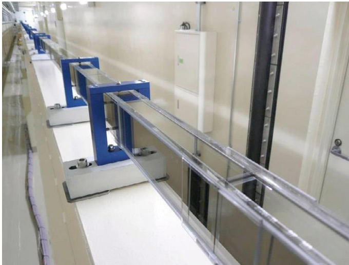
80m Guide for HRPD at J-PARC Fabricated by Swiss Neutronics
