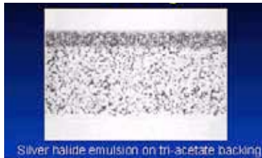
Silver halide emulsion on tri-acetate backing
